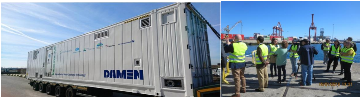
Test of "InvaSave" (1 st port BWT system certified by IMO) developed by
